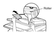
(C) If the original does not move easily into the exit area, remove it in the direction of the arrow while rotating the knob.
